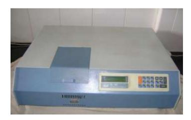
➤ Visible(Systronics-Make) & U/V Spectrophotometer (Double Beam Thermo Make): Spectrophotometers are useful in identification and determination of a sample. Many projects at degree, PG and research level can be performed with these instruments. Water and soil analysis can be performed.
